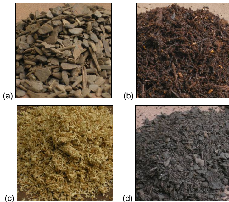
Figure 2. Organic materials: timber industry waste products (a) pine bark chips and (b) pine bark fines; (c) Sphagnum moss (saturated); (d) tree fern fibre.
